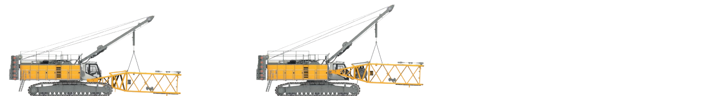
Assembly of boom foot
